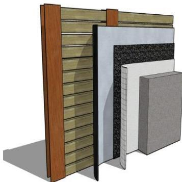
**MG-36 System** Blind side composite waterproofing system that combines a durable HDPE protection sheet, and a spray applied non-curing Polymer Rubber Gel that is encapsulated by a second LLDPE protection sheet used on new construction projects.
